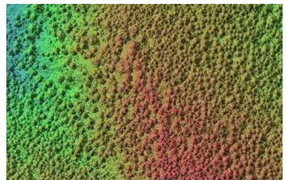
LIDAR virtual terrain displays of a forested area using all points (above) and using only ground points classified in TNTmips (below).
